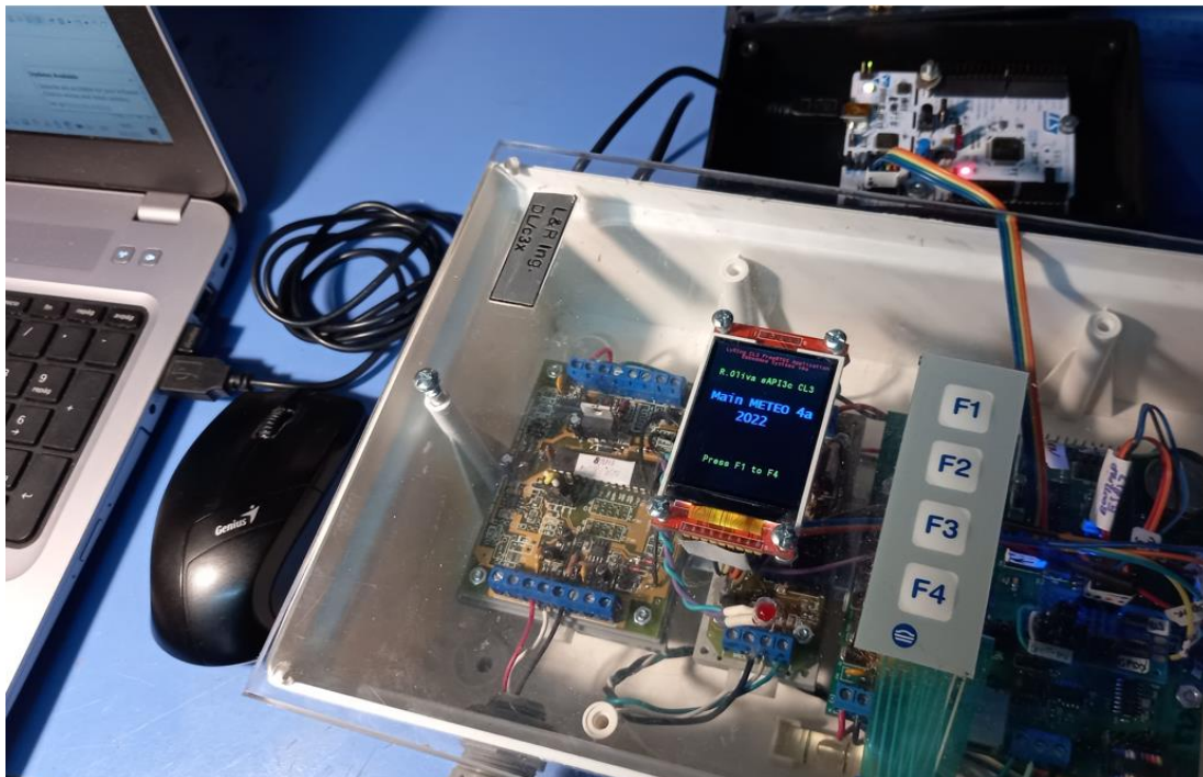
Figure 21 – Running Example 4 project with FreeRTOS on a CL3 board (right) connected to METEO board (left) thru an RS485 adapter (middle), with membrane Keyboard and ILI9341 display to the SPI port connector. The PC connects through the USB port to the STLink V2 debugger (top) and another USB port for the Terminal.
